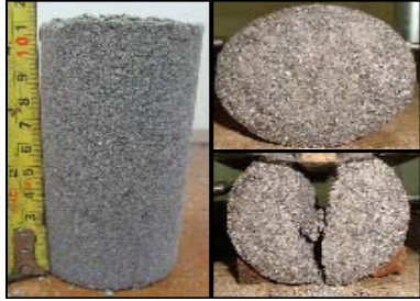
Gambar 5.1 benda uji diameter 50 mm campuran pasir, kapur, ASP
