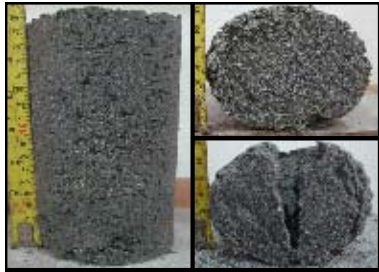
Gambar 5.3 benda uji diameter 70 mm campuran pasir, kapur, ASP
