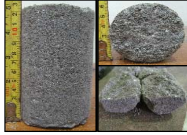
Gambar 5.2 benda uji diameter 60 mm campuran pasir, kapur, ASP
