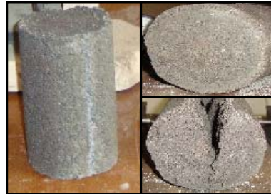
Gambar 5.4 benda uji diameter 90 mm campuran pasir, kapur, ASP
