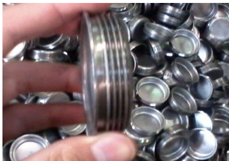
Gambar 1.5. Hasil proses thread rolling .
