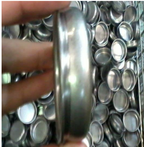
Gambar 1.4. Hasil proses collaring .
