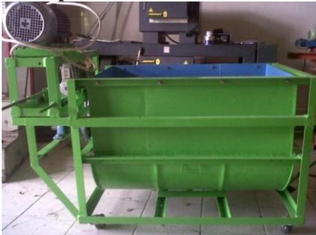
Gambar 3.1. Sling pump skala laboratorium
