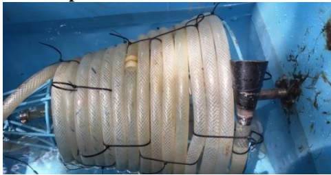
Gambar 3.1. Sling pump tipe kerucut skala laboratorium
