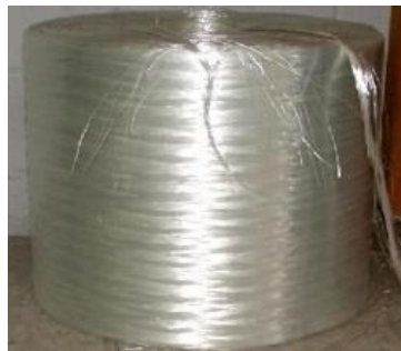
Gambar 2.5 Serat gelas roving
