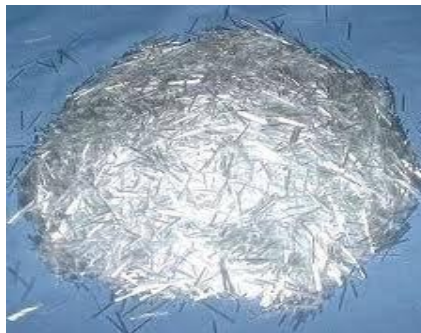
Gambar 2.7 Serat gelas chopped strand
