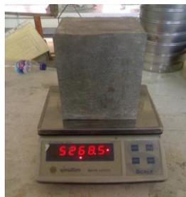
Gambar 4.13 Penimbangan beton geopolime
