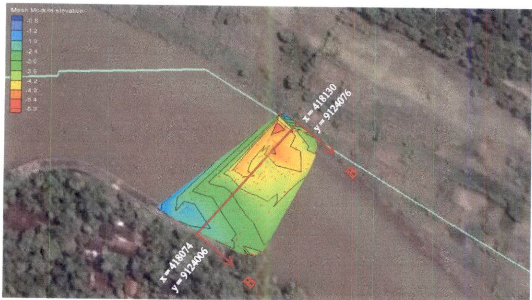
Gambar 5.4 Cross section B-B pias Intake Sapon menggunakan Aquaveo Surface Water Modeling System v10.1.8.
