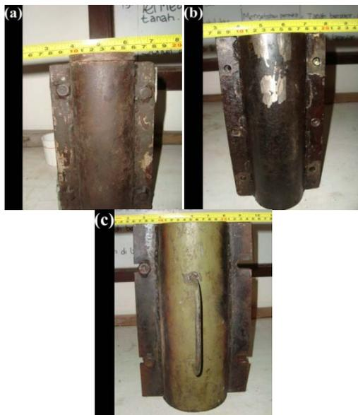
Gambar 4. Cetakan silinder berdiameter (a) 50 mm, (b) 70 mm, (c) 110 mm
