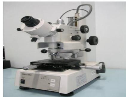
Gambar 3.3. Alat mikro Vickers
