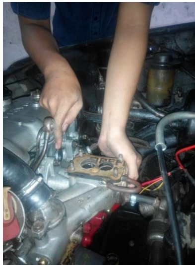
Gambar 5.14. Melepas Intake Manifold
