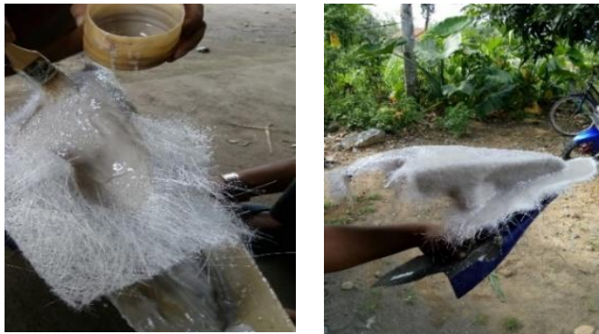
Gambar 4.9. proses hand lay up
