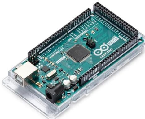
Gambar 2.6 Arduino Mega 2560
